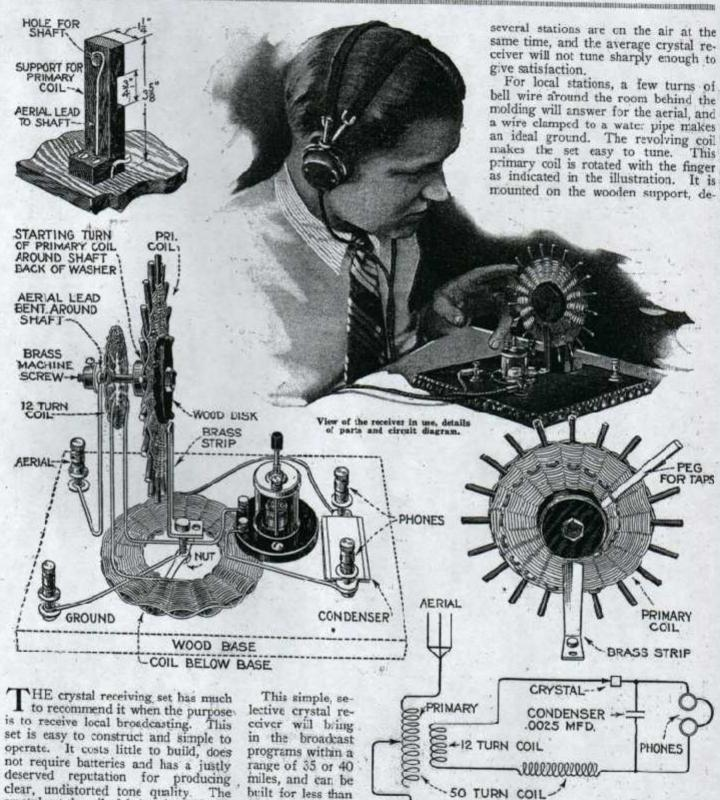
crystal set described below by Will H. Bates which appeared in Popular Mechanics magazine, has the additional advantage of being able to separate the "close together" stations, giving the sharp tuning usually obtainable only in vacuum tube sets.
