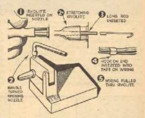
When the nozzle haives are in contact with one another, the flexible insulating tube can be easily slipped over their outer surfaces. Then, when the nozzle halves are separated, the mouth of the tube is stretched open.
