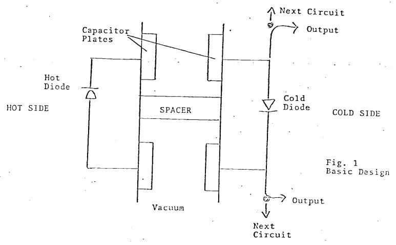
Typical power output from a single circuit is about  $10^{-6}$  watts. Consequently to achieve reasonable power output the circuits need to be tightly spaced. The inventor states that the density needs to be between  $10^6$  and  $10^{10}$  devices/cm<sup>2</sup>. Below  $10^6$  devices/cm<sup>2</sup> the efficiency is unreasonable. Above  $10^{10}$  devices/cm<sup>2</sup> the linear dimensions approach the mean free path of an electron. Table 1 shows the consequences of the circuit density.
