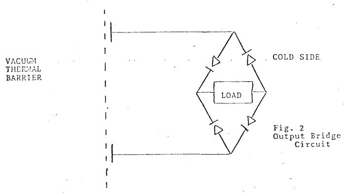
For electrical engineers who understand diodes as circuit elements better than as quantum mechanical devices, Figure 2 provides a more appealing conceptual explanation of how rectification can occur. With the above exceptions, the majority of experts felt that, in principle, the concept of rectification of thermal noise power was theoretically valid.
