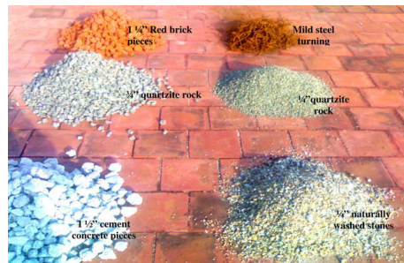
Figure 20. Materials employed in the experiential study. Reprinted with permission from Ref. [44]. Copyright 2010, Elsevier.
