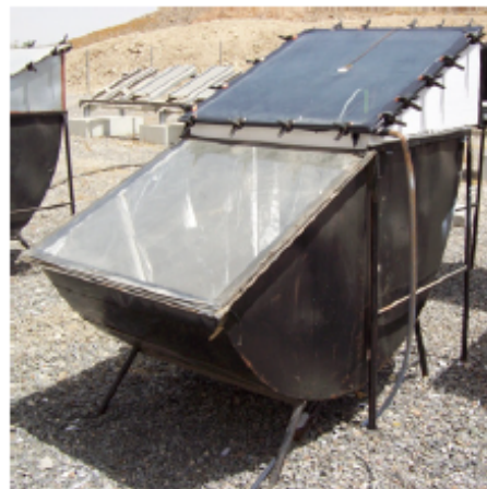
Figure 41. Schematic representation of an inverted absorber solar still system for optimized productivity and water depth efficiency. Reprinted with permission from Ref. [75]. Copyright 2011, Elsevier.
