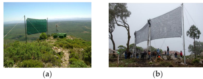
Figure 3. Different types of fog harvesting systems. (a) LFC fog collector situated at Mount Machos (Spain) [34]. (b) LFC fog collector situated at Guatemala [44].
