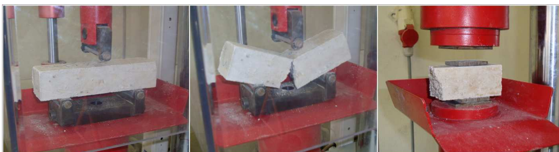
Fig. 1: a) and b) to flexural strength and c) to compressive strength tests
