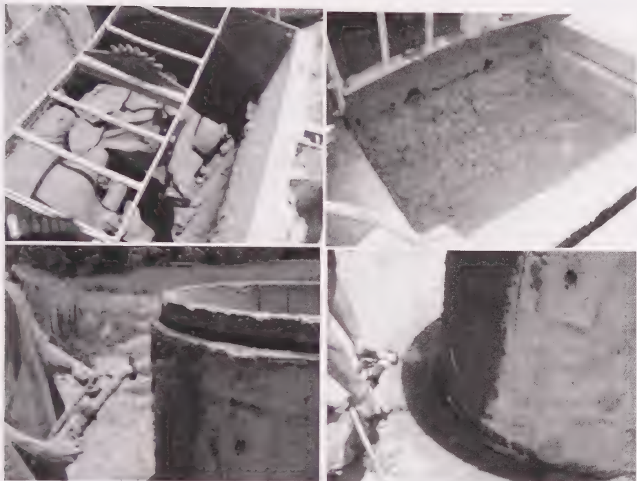
FIG. 9— Mixing and spraying during a sprayable geopolymer field test.
