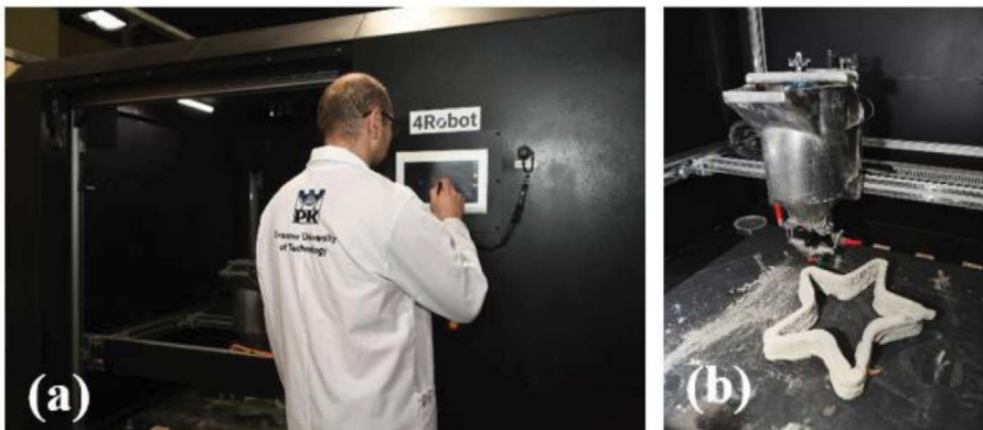
FIGURE 5.6 Photos from the project realisation: (a) programming of 3D printer and (b) nozzle and exemplar element.
