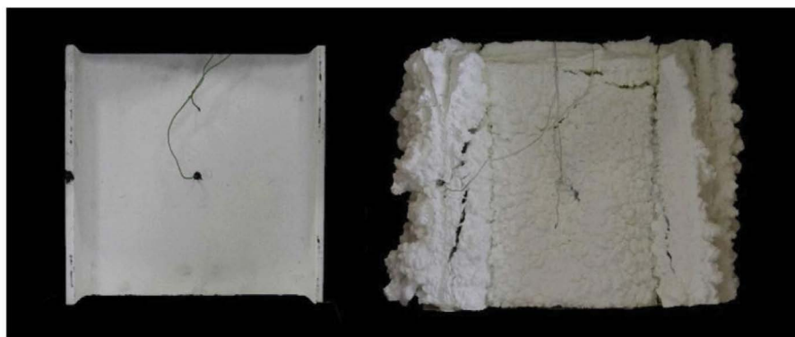
FIGURE 7.1 Steel structure protected with an intumescent coating before (left) and after (right) fire test. (Reprinted with permission from ref. [3]. Copyright 2019 Elsevier and [24].)
