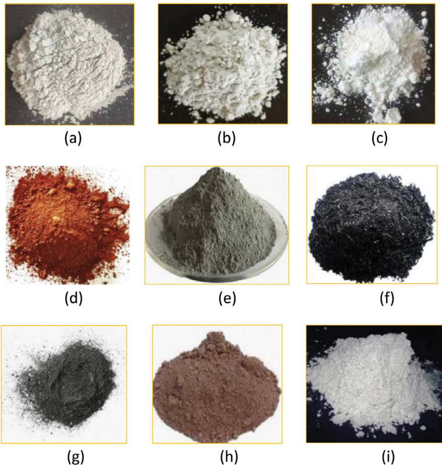
FIGURE 1.4 Particle images of (a) FA, (b) GGBS, (c) MK, (d) RM, (e) SF, (f) RHA, (g) volcanic ash, (h) calcined clay, and (i) diatomaceous earth.
