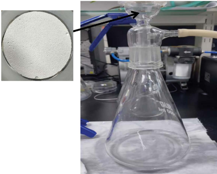
FIGURE 10.9 Test design for geopolymer membrane.
