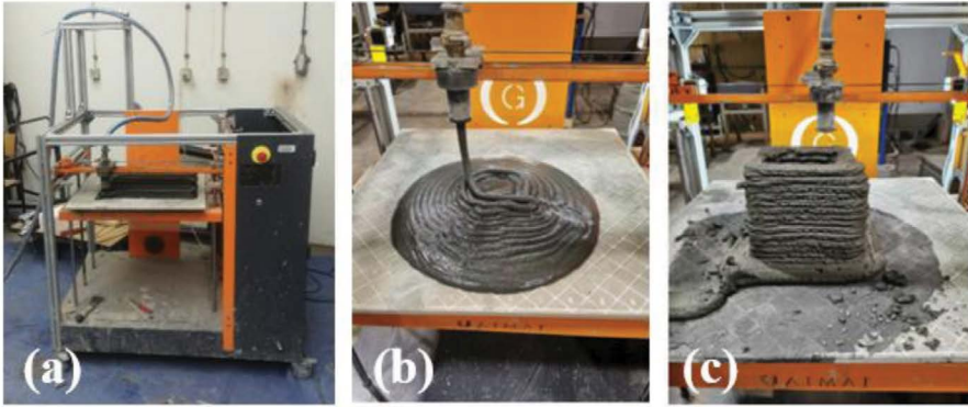
FIGURE 5.4 Photos from the project realisation: (a) used 3D printer, (b) problems with the liquidity of geopolymer paste, and (c) 3D printing process for exemplary element.
