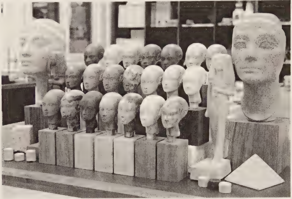
Figure 1.1: Samples of moulded geopolymer stones (limestone, granite, sandstone, arkose, ...) (2003).
