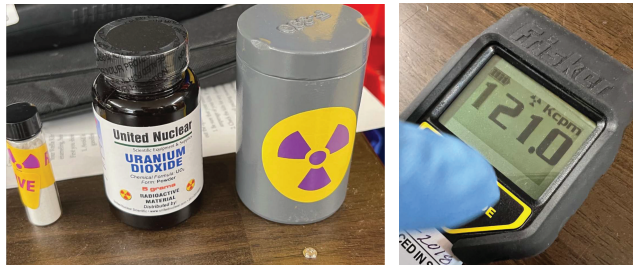
(a) Radioactive Nuclides: ThO 2 , UO 2 , Am (b) Beta ray counting (121 kcpm)
