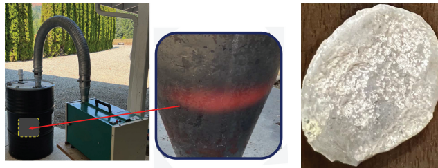
(c) Neutralization test setup used for the neutralization test, showing the heated layer inside the container (the area that has turned red) and thermite reaction products.
