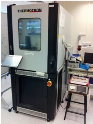
Fig. 6.3 Thermotron SE-300 enclosed chamber to monitor behavior of composite materials under controlled temperature and humidity
