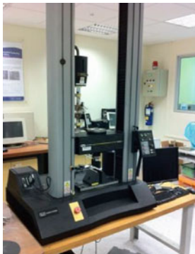
Fig. 5.3 Specifications of Instron 5569 universal testing machine used in the compression experiments of the composites
