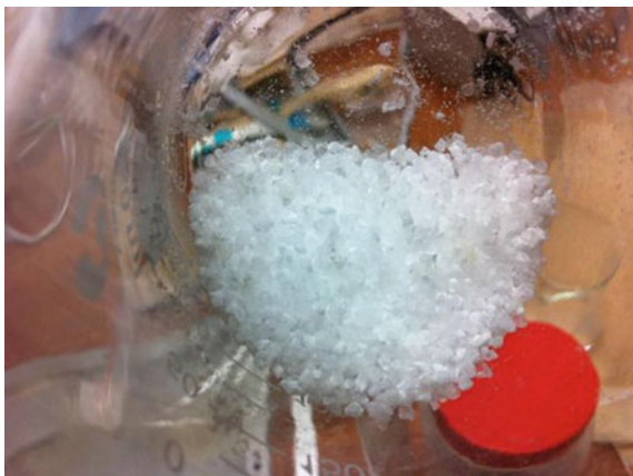
Fig. 4.1 Non-binding of heat-treated aerogels with gelatin. Aqueous gelatin solution failed to bind with heat-treated silica aerogel granules but was instead absorbed by the aerogels as an indication of loss of hydrophobic properties
