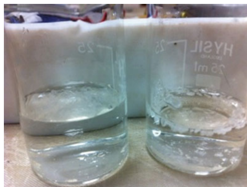
Fig. 3.2 Loss of hydrophobic properties in silica aerogel granules. Left Beaker Unheated hydrophobic aerogels are seen floating on the surface of the water. Right Beaker Heated aerogels turned whitish indicating shrinkage in volume due to infiltration of water into the pores. As a result, the aerogels become denser and settle down at the bottom of the beaker
